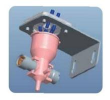
Improved DC impedance technology is used to count and size the RBC and PLT. The smaller counting aperture (50  $\mu$ m in diameter) provides better performance on samples with low PLT.
